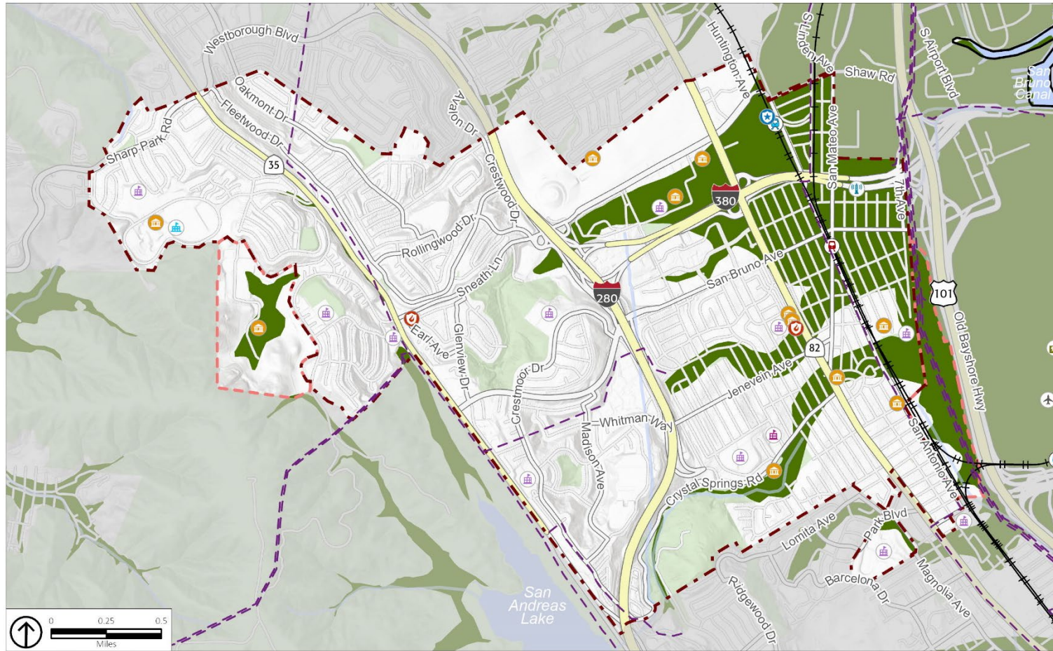
Figure 7: Liquefaction Hazard Areas
