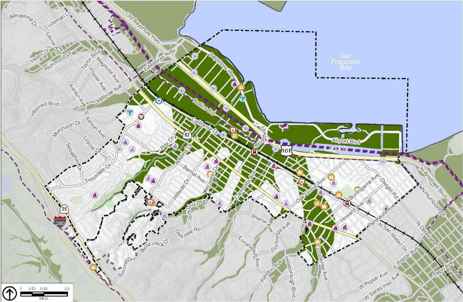
Figure 7: Liquefaction Hazard Areas
